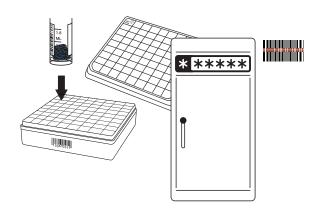
4. Scan bar-code on the cryovial and box to your software. Store inoculated cryovial in the cryobox at selected temperature.
