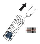
1. Remove cryovial from freezer and scan barcode. Aseptically remove a single bead with a sterile needle.
