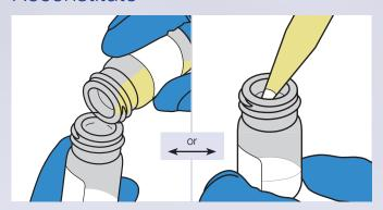
Reconstitute the pellet by transferring the entire contents of vial RB into vial PEL.
