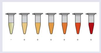
Record the colour of the test solution immediately or up to 20 minutes after incubation.
