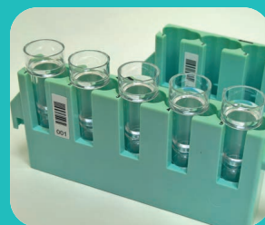
Automatic standard dilution for calibration
