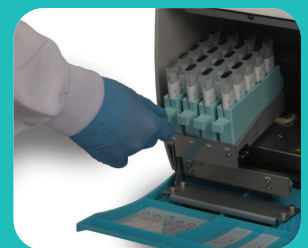
Analyse up to 20 samples at a time, 5 per rack
