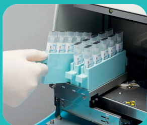
Random access gives a sample throughput of 88 tests/hour
