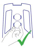
Insert capsule into retaining clip in canister.
