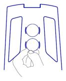
Remove silica gel capsule by lifting from behind.
