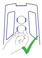
Insert capsule into retaining clip in canister.
